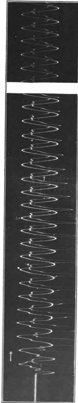
Fig. 30. — cd10075. — Transient Starting Current of Alternating-current Transformer. 20 Cycles Later.
